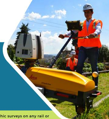
Independent positioning system for high resolution 3D topographic surveys on any rail or metro track. Resolution surveys in three dimensions on any railway or metro track. It is equipped with GPS, laser meters (DMI) and Inertial Measurement Units (DMU) that allow positioning even without access to GPS signal.
